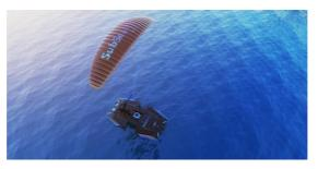
SubSea RO Wind – technology to desalinate seawater into freshwater. Source: Hydro Wind Energy Hydro Wind Energy is currently in the midst of a project building and testing a subscale system of both technologies off the coast of Fujairah in the United Arab Emirates with several offshore engineering firms and strategic partners.
